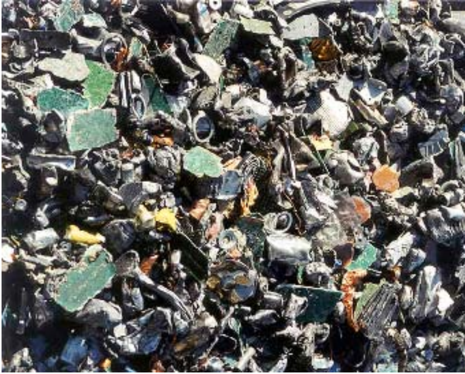
D) Metal fraction after Eddy Current Separator I
